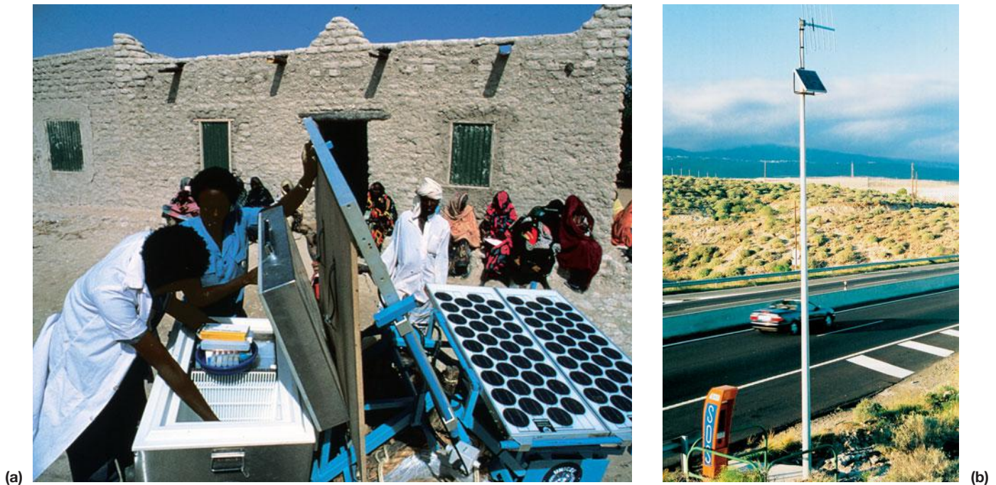
FIGURE 16.7 (a) Panels of photovoltaic cells are used here to power a small refrigerator to keep vaccines cool. The unit is designed to be carried by camels to remote areas in Chad. (b) Photovoltaics are used to power emergency telephones along a highway on the island of Tenerife in the Canary Islands. [Source: (a) H. Gruyaeart/Magnum Photos. Inc. (b) Ed Keller]
