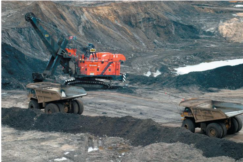
FIGURE 15.18 Mining tar sands north of Fort McMurray in Alberta, Canada. The large shovel-bucket holds about 100 tons of tar sand. It takes about two tons of tar sand to produce one barrel of oil.
