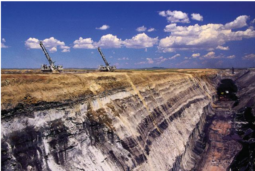
FIGURE 15.14 Strip coal mine in Wyoming. The land in the foreground is being mined, and the green land in the background has been reclaimed after mining.
