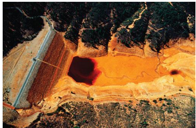
FIGURE 19.8 Aerial view of an acid mine drainage holding pond adjacent to an iron mine (located in the mountains of southwestern Colorado).
